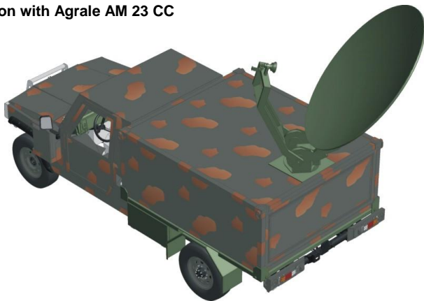
S-394 integrated with a satellite communications system and Agrale Marrua AM 23 CC
