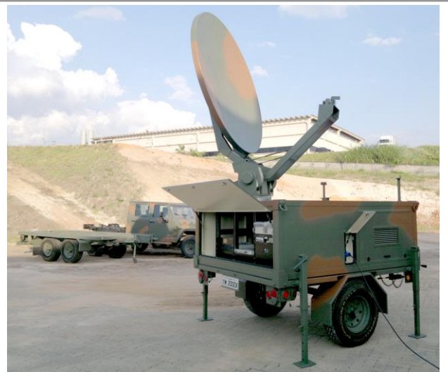
S-394 integrated to a HMT-2000 semi-trailer and satellite communication
