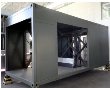
Steel Shelter for Radar Syst. Integration
