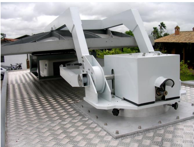
RF COM Manual System: Elevation adjustment is made through a hand crank with reduction gears. Azimuth is adjusted by manually rotating the antenna on the rotatable base.
