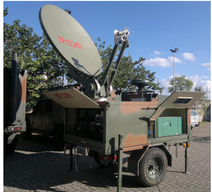
SAT-2000A integrated with positioner and automatic controller, UPS and power distribution, diesel generator with auxilliary external fuel tank, air conditioning, and equipment racks on a HMT-2000
