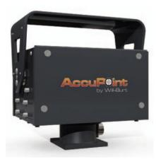
AccuPoint positioners are designed to deliver maximum performance for top-of-the-mast antenna positioning. The AP-100 is a 100 pound (45 kilograms) payload capacity positioner. Design highlights feature optimized gear and motor ratios for enhanced performance and easily accessible, adjustable-limit cams for easy service. The AP-100 features an easy to replace breakaway base with lanyard for added safety.
