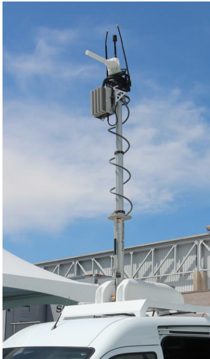
NS with Accupoint microwave antenna positioner and radio support. (see more details in the Accupoint page in this catalog)
