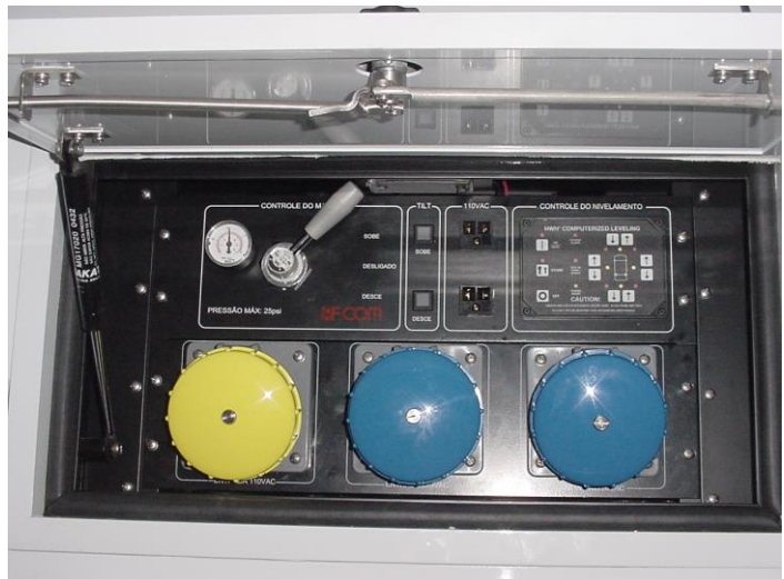
Energy connections panel, leveling commands and masts.
