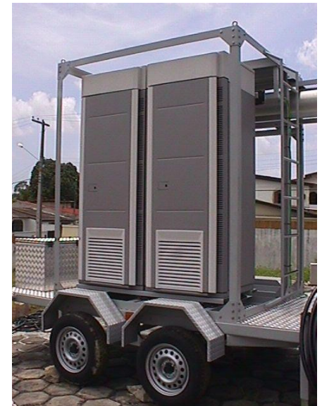
With 18.3m mast and Nokia Ultrasite BTS
