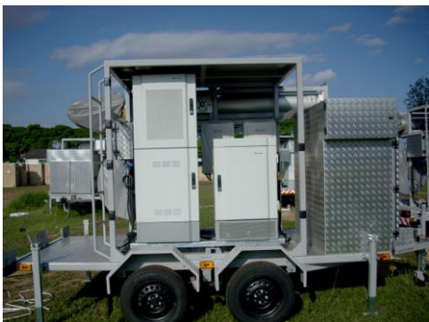
With 18.3m mast and Huawei 3G BTS
