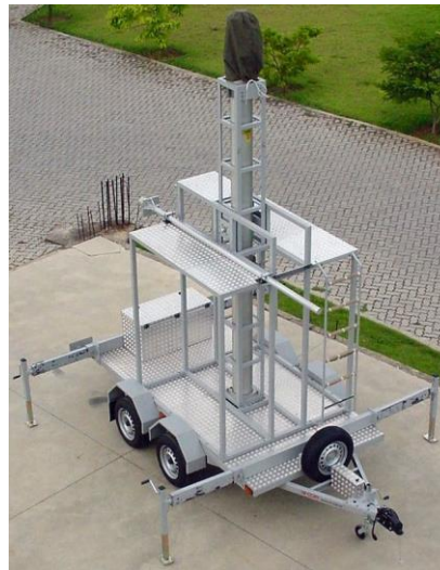
With 24.3m mast and extensible stabilizer arms
