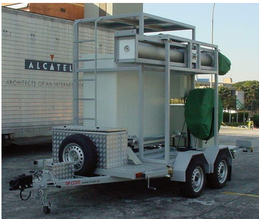
With 18.3m mast and Alcatel BTS
