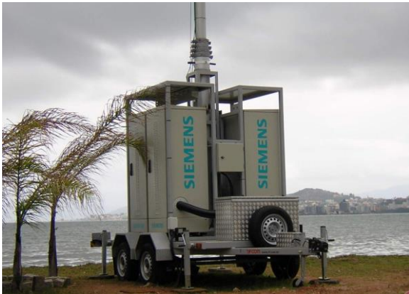
With 18.3m mast and Siemens BTS
