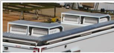
Roof Top Capacities: 13.5 kBTU, 15 kBTU and 15 kBTU + Heat Pump Option: Rugged (no Heat Pump)
