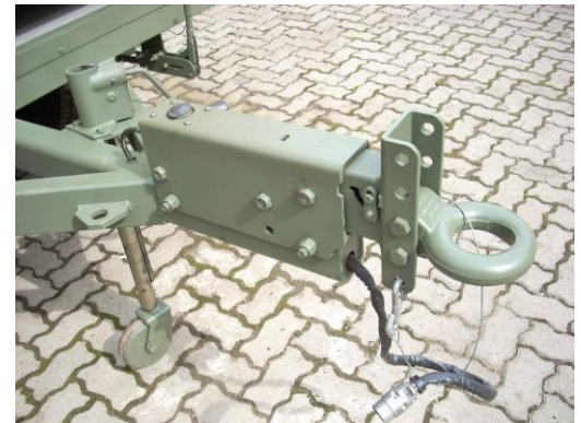
Inertial braking system and pintle ring (lunette eye) hitch
